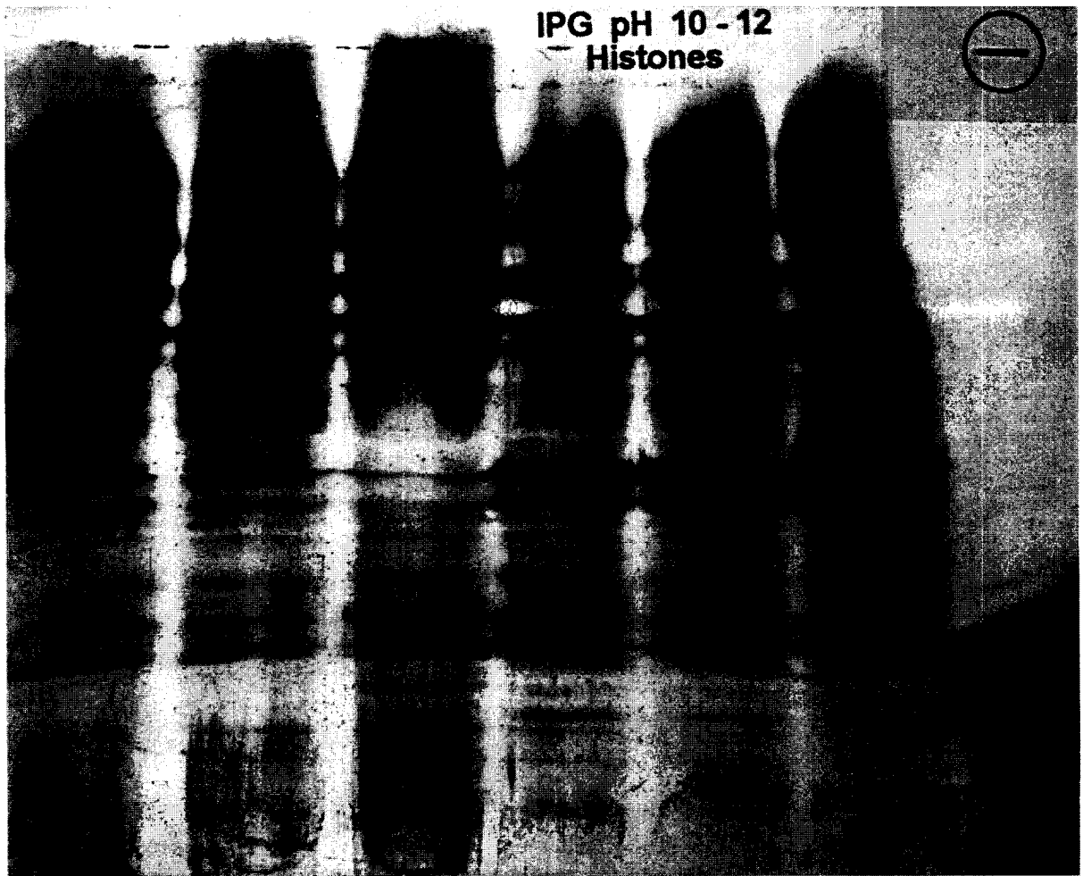
Fig. 6. Focusing of histones in an IPG pH 10–12 interval. Gel: 6% T, 4% C polyacrylamide matrix, containing an IPG 10–12 gradient, reswollen in 7 M urea, 1.5% Nonidet P-40 and 0.5% Ampholine pH 9–11. The gel was run at 10°C under a layer of light paraffin oil at 500 V for the first hour, followed by increasing voltage gradients, after sample penetration, up to 1300 V for a total of 4 h. The samples (2 mg/ml; 50 \mu l seeded) were loaded in plastic wells at the anodic gel surface. Staining with Coomassie Brilliant Blue R-250 in \text{Cu}^{2+} . Tracks (from left to right): (1–3) VIII-S histones; (4–6) II-AS histones; (7) cytochrome c (the main upper band has a pI of 10.5). Note the fine spectrum of sharp bands (more than a dozen) focusing in the pH 10–11 region (from Bossi et al. [63]. with permission).
